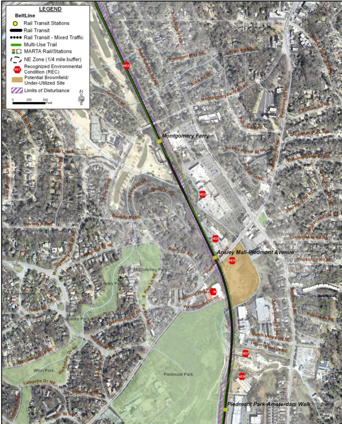
Figure 4-26: Hazardous Materials Sites (Montgomery Ferry/Ansley Area)
